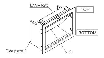
Do not leave any gap between the flap lid body and the mounting surface.
